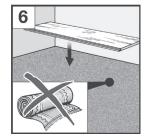
Carpeting, foamed PVC floor coverings and all types of foam must always be removed [6] as they are not suitable as subsurfaces. Walking on the floor surface may otherwise cause a springy movement in the flooring and too much pressure in the edge areas, which can result in the formation of gaps. Carpeting must also be removed for hygienic reasons. Moisture can lead to the formation of mould and bacteria.
