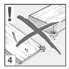
The subsurface on which the panels are to be installed must enable the floor panels to be installed in accordance with the manufacturer's instructions (product insert). Mineral subsurfaces (e.g. screed, water-based heated screed, concrete, asphalt) count among the suitable subsurfaces. Please note that substructures must comply with the generally recognised rules for dry constructions in wet rooms.
