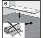
Carpeting, foamed PVC floor coverings and all types of foam must always be removed [6] as they are not suitable as subsurfaces. Walking on the floor surface may otherwise cause a springy movement in the flooring and too much pressure in the edge areas, which can result in the formation of gaps. Carpeting must also be removed for
